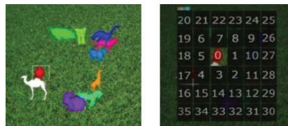
Fig. 4. A ClickAnimal image (left) and 6 \times 6 grid (right) determined by red turkey's bounding rectangle.
